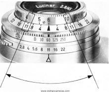
The scale (11) bears two sets of figures opposite the distance scale. The figures on the distance scale opposite each set of identical aperture figures denote the beginning and the end of the depth of field. Example: setting 6 ft at aperture f/11; the depth of field will cover the zone between 4 ft and 10 ft. Exact values are given in the table on the reverse of the instruction booklet.
