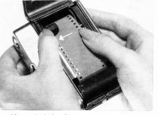
Now wind the film on to the take-up spool until the transport sprocket (15) engages the perforations on both sides. The cut-out knob (17) should be depressed to facilitate this operation. Replace the camera back and lock it.
